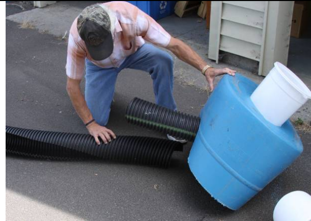
Figure 23. Test fitting the tunnel section into the collar. The final attachment of the tunnel to the collar and nest chamber is done in the field, after the hole has been dug and the nest chamber has been placed into it.
