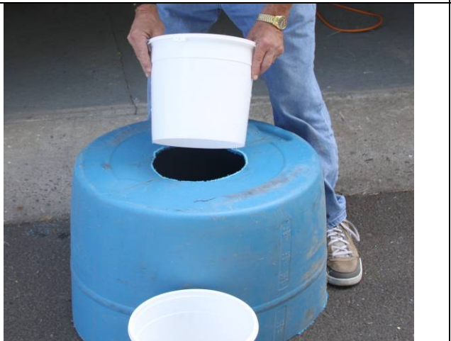
Figure 16. Bottomless pail fits into barrel top.
