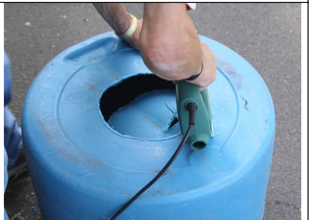
Figure 14. Use jigsaw to cut hole for pail to just slip about 1 in. into barrel.
