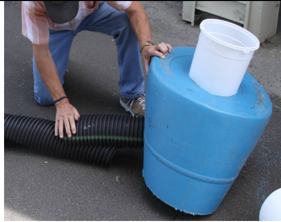
Figure 24. Test fitting (continued). It is important that the main tunnel be placed on the inside of the collar, to aid in future operations of the burrow system. Main tunnel should fit 2-3 rings inside the main barrel chamber. No caulking is used to attach main tunnel section to collar/nest chamber.
