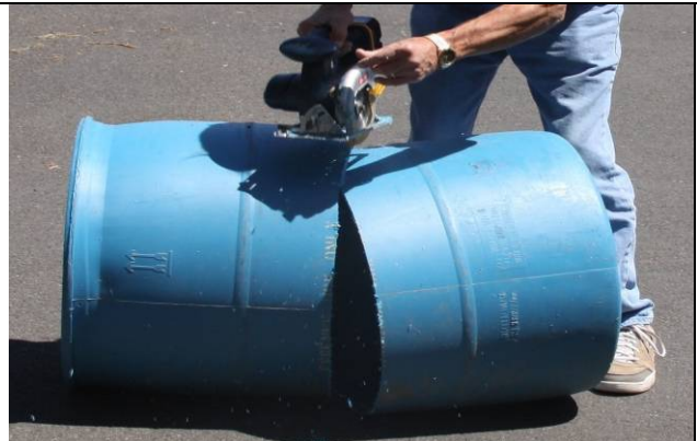
Figure 12. Cutting barrel in half with skill saw.
