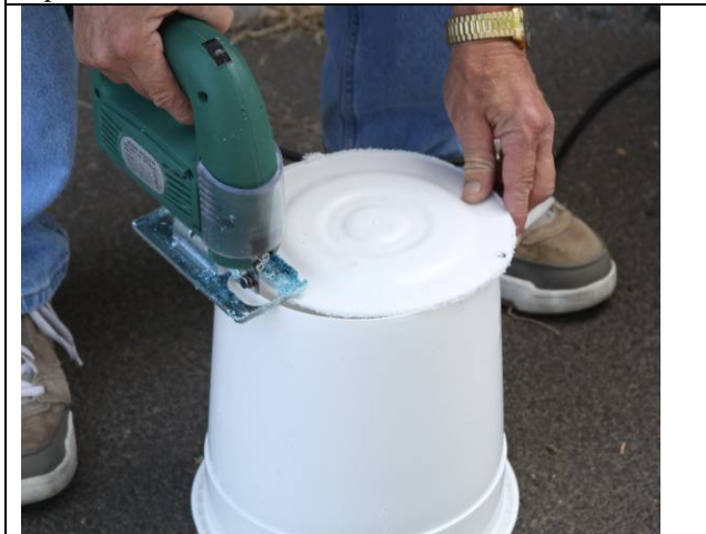
Figure 15. Use jigsaw to cut bottom out of one 2.5 gallon pail.
