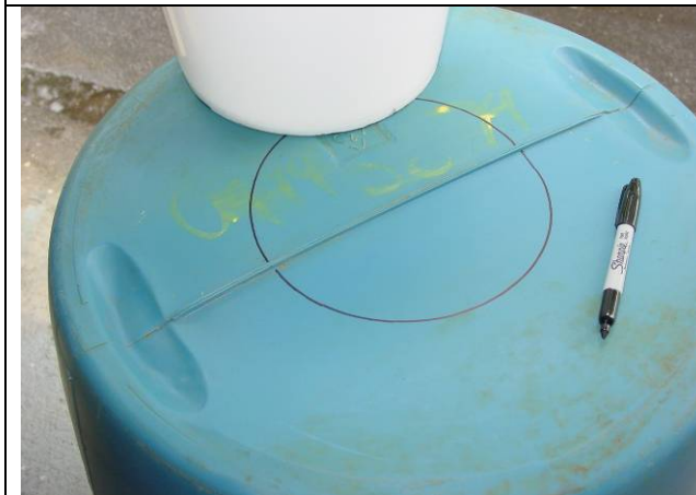
Figure 13. Trace outline of 2.5 gallon pail bottom onto top of barrel section.
